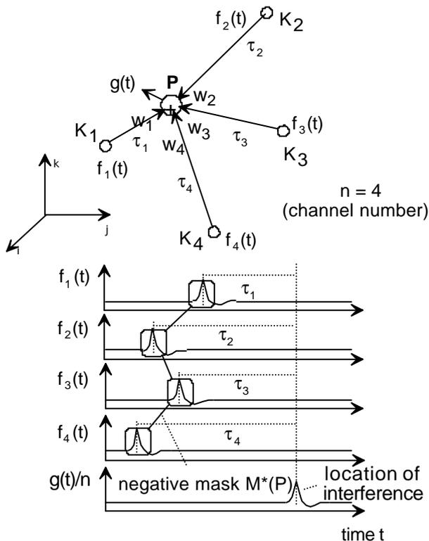
Fig. 2: A receiving, negative delay vector  $M^*$  of  $P$
