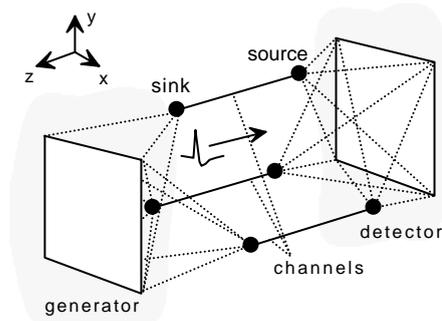
**Fig. 7: Experimental field PSI-Tools. Black pixels of a bitmap act as signal generators, producing time functions. Channel sinks sum up all time functions of the generator field. Source points send the waves to detector field(s). INI-files save velocities, co-ordinates, time-functions of black pixels.**
