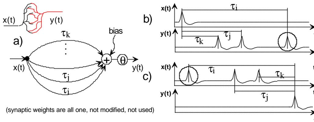
**Fig. 3) Basic functions of a neuron or a neural group a) Circuit structure, b) Burst generation with low bias, c) Burst detection with high bias**
