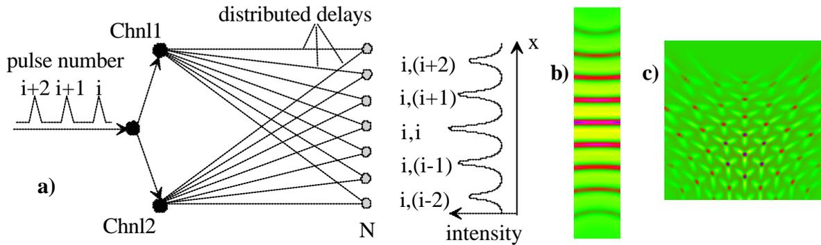
**Fig. 5) Frequency maps. a) Two channel circuit example, b) simulation result c) spatial code of a frequency - three channel wave interference simulation result.**
