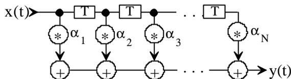
Fig. 10) Digital FIR-filter as modified IN
