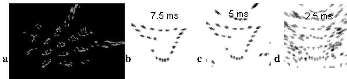
**Fig. 7) 3-channel pulse-wave projection of a "G". a) Cross interference residua around a self interference figure (BIS2000). Cross interference overflow produced by higher fire rates b), c), d) with average fire delay in milliseconds**
