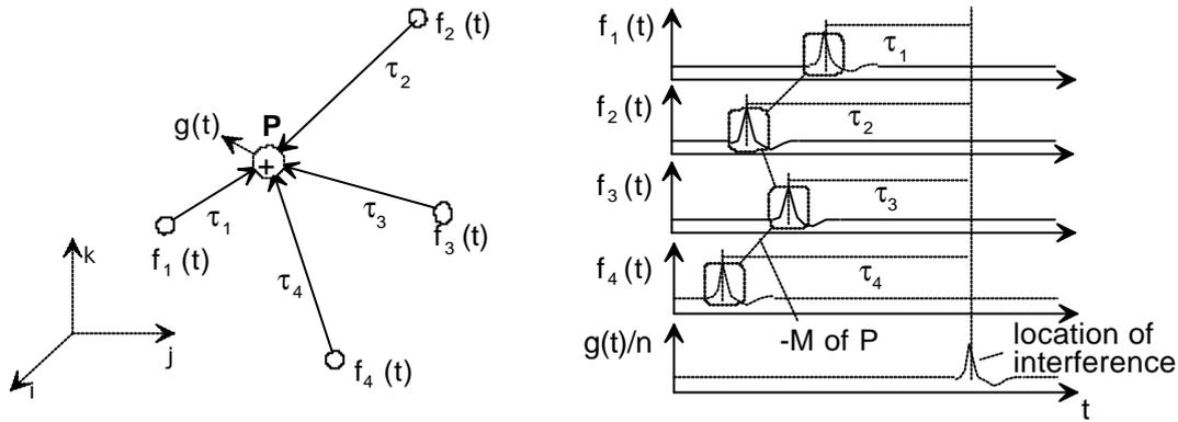
**Fig. 1) Example: Time function  $g(t)$  of point  $P$  summing four sources  $f_k(t)$**
